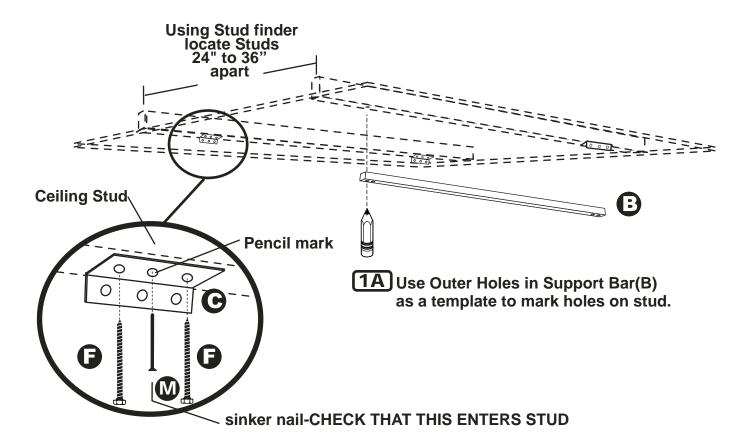
1B Attach Angles(C) into Ceiling Studs.
