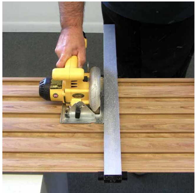
Saw cuts are quick and clean. This cut is with storeWALL "good side down" for a perfectly clean face edge.
