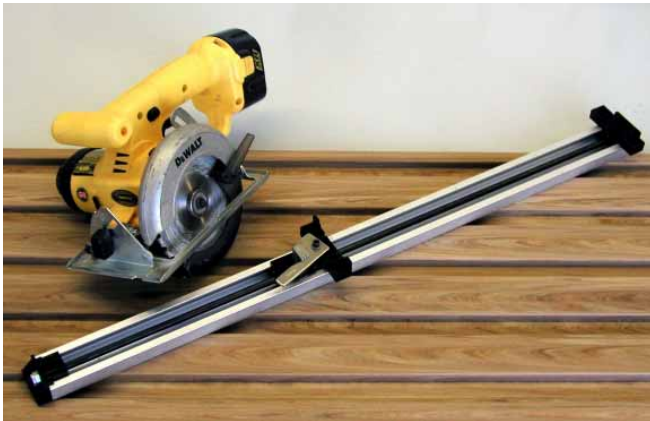
Tru-Grip straight edge with width adjustment and clamp.
